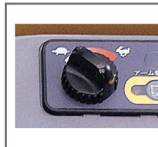
Rotary Engine Throttle with Auto Idling System
